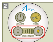
2 Set the required luminosity with 5 dimming levels.
