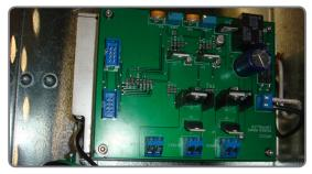
The power supply generates 24V from 100 – 240 VAC for each solenoid. There are three (3) connections (1 per solenoid) and two (2) connections (1 per each electric brake handle).
