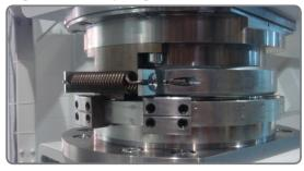
The springs generate friction by pulling the brake shoes towards the center drum, preventing the bearing from rotating freely.
