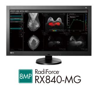
Multi-modality monitor for simultaneously viewing multiple medical images such as digital mammography, magnetic resonance imaging (MRI), and ultrasound images all on one unobstructed screen. Industry first multi-modality color widescreen monitor to receive FDA 510(k) clearance for mammography and general radiography.
