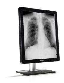
Equipped with high-bright LED backlights, Barco's Coronis 5MP LED renders more JNDs (Just Noticeable Differences) to help you see more shades of gray. Additionally, Per Pixel Uniformity ensures every pixel is DICOM-compliant at all times, which increases contrast to noise ratio. Subtle details become more noticeable more quickly, resulting in reduced windowing and leveling time.
